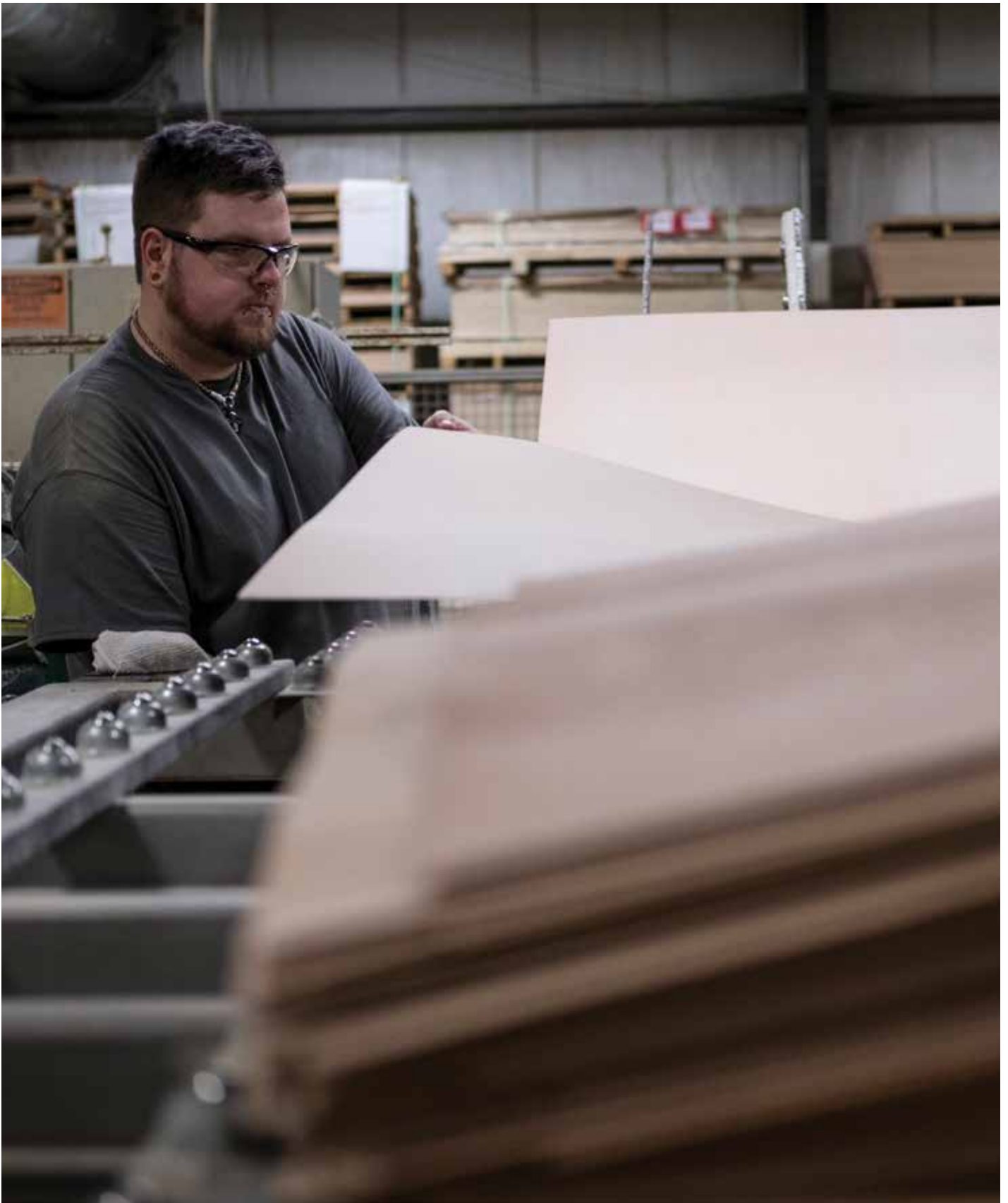
Face veneer is pulled from a stack of veneer as part of the manufacturing process. Having the right cut of veneer with face style and color sets the tone for what awaits beyond the door.
