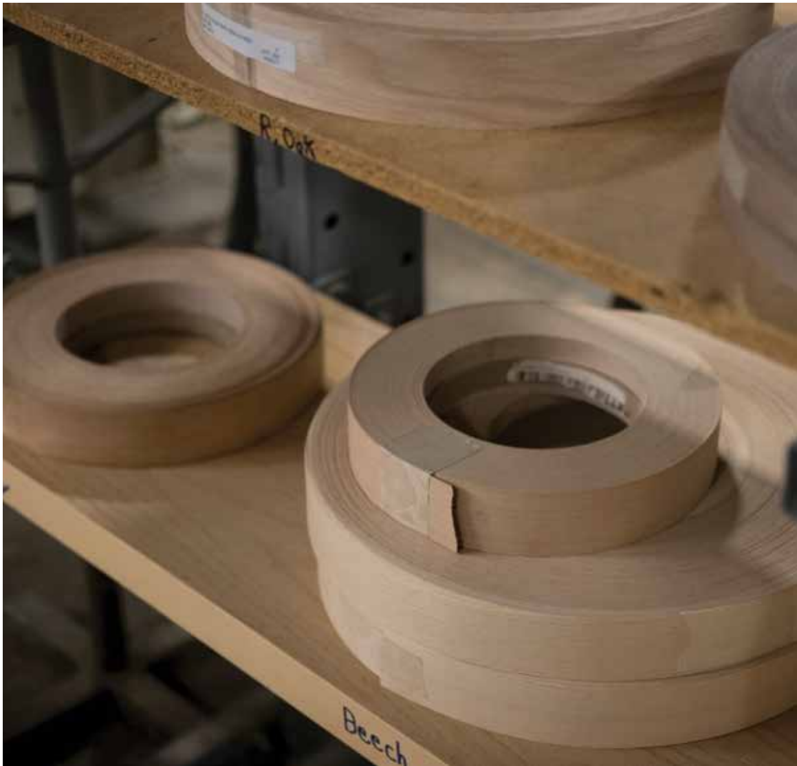
Rolls of veneer edge banding from a few of the hundreds of different species of wood that can be used in the construction of wood doors. Two of the more popular species are birch and red oak.
