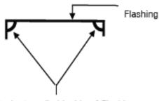
Sealant applied inside of Flashing prior to installation of door along both sides and across each end
