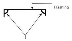
Sealant applied inside of Flashing prior to installation of door along both sides and across each end
